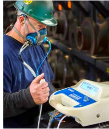
Controlled Negative Pressure - OHD® Quantifit® CNP using the REDON method being used to conduct a Quantitative Fit Test (QNFT) upon a subject wearing a half face facepiece respirator. Image: courtesy of OHD®
