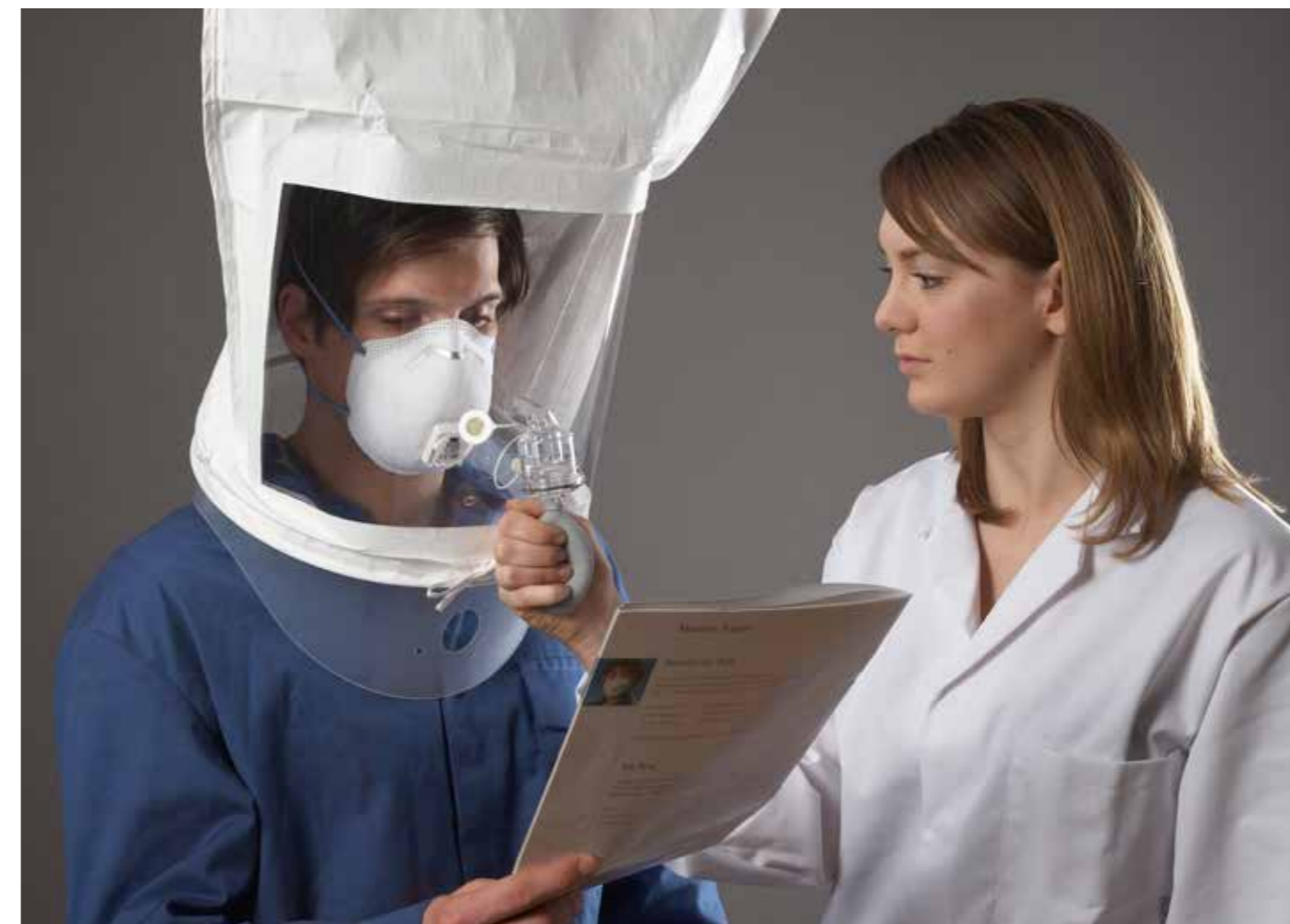
Figure 1 - 3M FT-30 Bitrex ® Fit Test kit being used to conduct a Qualitative Fit Test (QLFT) upon a subject wearing a disposable facepiece respirator
