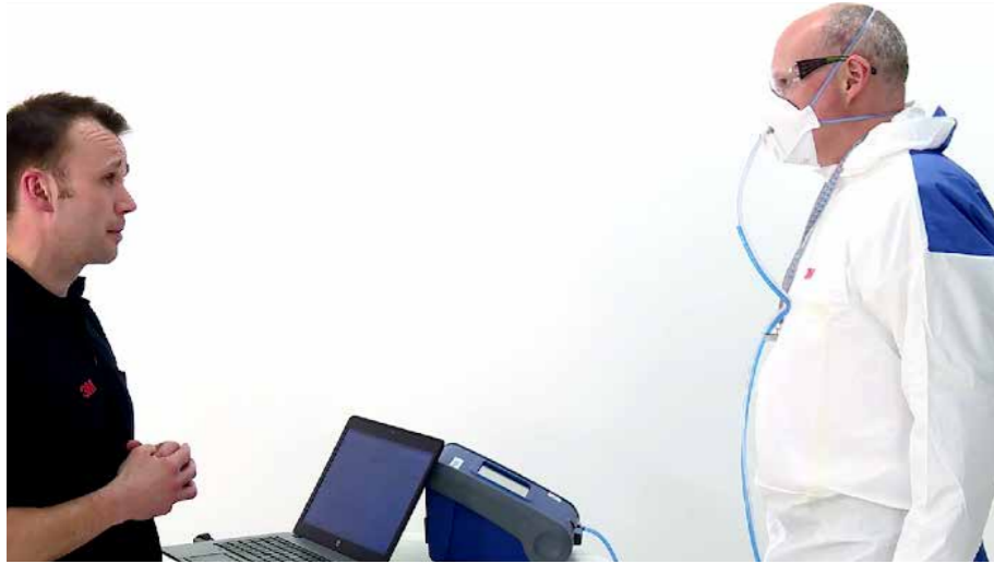
Figure 2 - Ambient Particle Counting - TSI® PortaCount® Model 8038 being used to conduct a Quantitative Fit Test (QNFT) upon a subject wearing a disposable facepiece respirator
