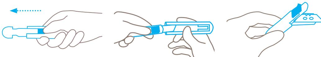
Use the slider to push the plastic insert back and out of the handle. Don't pull the insert while holding onto the slider. Reverse or replace the blade and reinstall the plastic insert. Make sure you position the new or turned blade exactly over the locating lugs.
