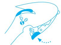
Finally, close the blade cover and push the blade holder **back into the handle**. With a click, everything is in place.
