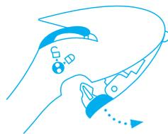
With two fingers, **disengage the blade holder** and swing it open.
