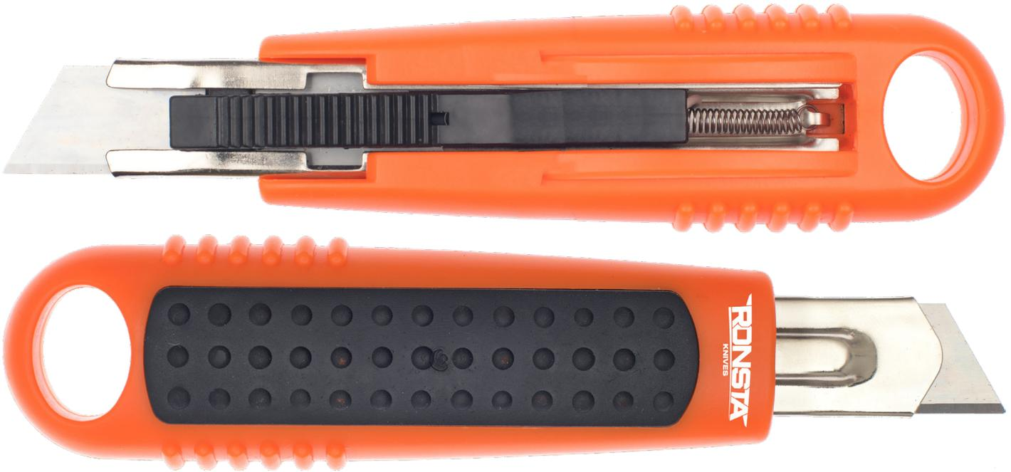
The KS004 side-slide safety knife is an economical cutter for a variety of applications. Offering a single-spring safety technology, this knife automatically retracts once the side trigger is released. The rubber dimple pad ensures a positive grip. The Japanese Sk-5 blade means a clean cut and is extremely durable. When used properly, this knife can reduce injuries in your workplace.
