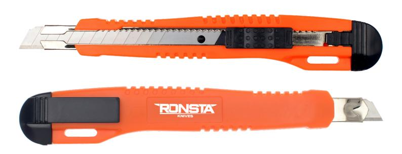
The economy 9mm snap blade knife performs a multitude of basic cutting applications. The smaller blade allows better control over the cutting surface. Once a blade becomes dull, you can snap the old segment away producing a new cutting edge. The black slide mechanism allows the blade to be secured in place by separating the slider.
