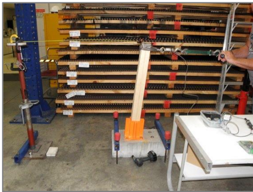
FIG. A1 POST IN CONCRETE INSTALLATION OUTWARD 1200N LOAD TEST
