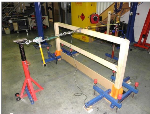
FIG. A5 TOP RAIL OUTWARD LOAD TEST
