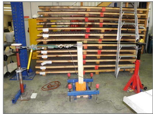
FIG. A2 POST IN PLYWOOD WITH BACKING TIMBER INSTALLATION INWARD 600N LOAD TEST
